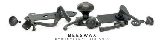
Beeswax is the most authentic finish for steel. After forging, the colours in the steel range from blue to deep red ochre. To preserve these colours, our products are dipped into hot beeswax which gives a subtle, matt richness and offers excellent protection when the products are fitted internally. An extremely natural finish and a far softer alternative to a black powder coated finish.
